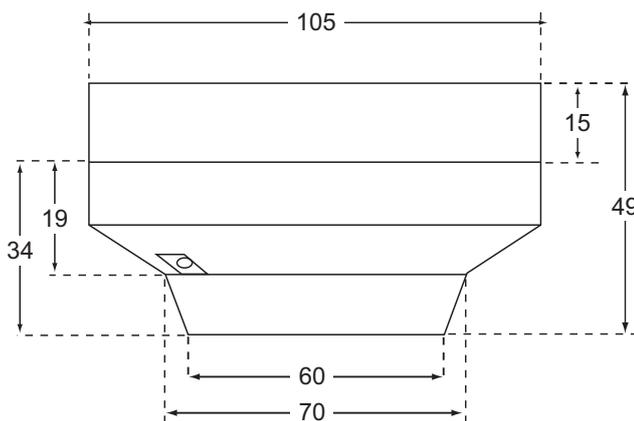
Montage: 2 x M4 Schrauben, 50/60/70 mm c/c
